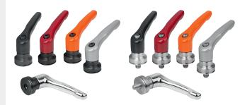
K1597 Fiberglass reinforced plastic handle, with steel clamping force intensifier. Internal or external threads, metric. Steel parts have black oxide finish.
