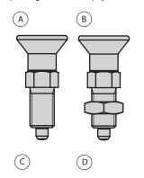
**Style A:** Non-lockout type, without locknut.
