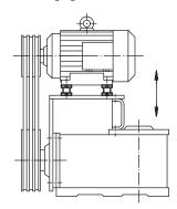
**Leveling Sets, low version** are designed for finer adjustments with a smaller range of travel. Ideal applications include adjustment of bearings, motors, drive components, and production lines. The primary difference of this product group is its low profile.
