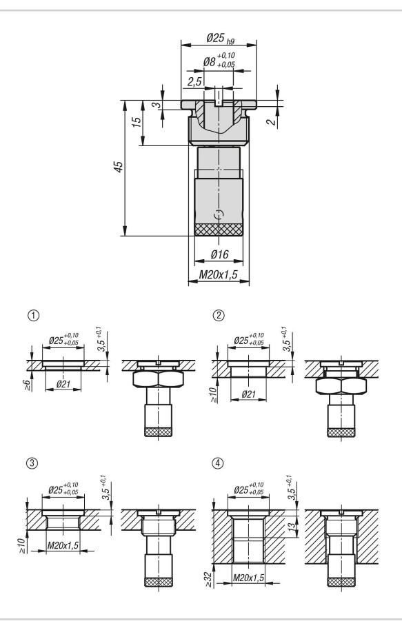
Ball lock bushings with twist lock
