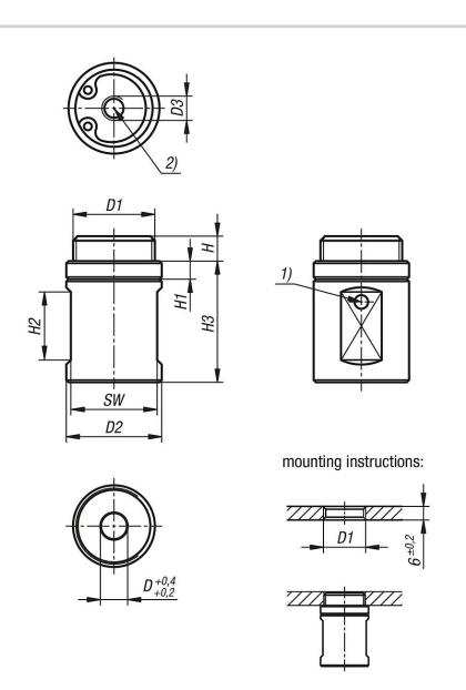
Locating adapters, cylindrical, stainless steel, pneumatic
